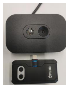
Fig.2 FLIR ONE dual camera and our designed dual camera with RGB and with infrared thermopile array
